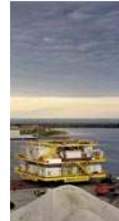
Wind turbine foundations for alpha ventus are shipped into Wilhelmshaven – each weighs 700 tons.
