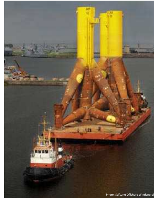
Wind turbine foundations for alpha ventus are shipped into Wilhelmshaven – each weighs 700 tons.
